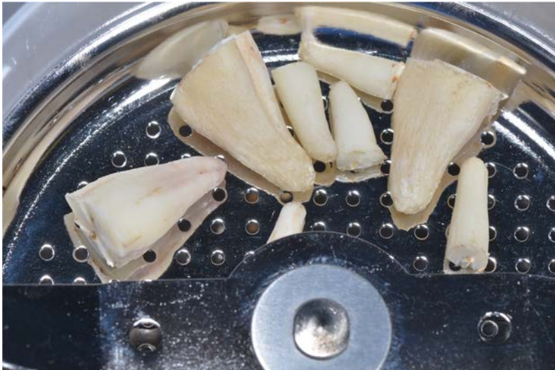
Fig. 2. Smart dentin grinder chamber with roots extracted from the dog.
